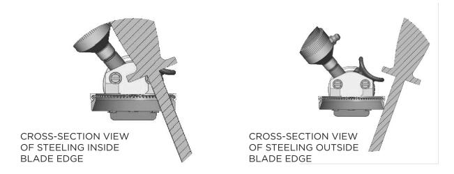
The INSIDE edge of the blade should be steeled only with the Special Steeling Device mounted on the inside diameter of the blade housing. This is accomplished as follows:
